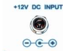
Fig. 9.3 External DC power connector
