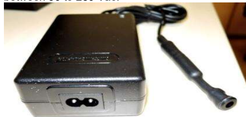
Fig. 9.4 Accumulator charger with adapted connector for accumulator plug (right) and socket for mains cable (left)
