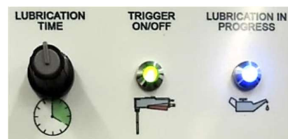
Fig. 8.3 Lubrication in progress
