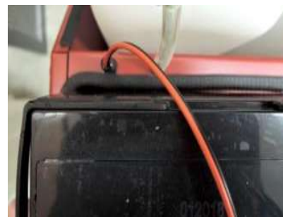
Fig. 9.2 Powering of Lubrico by accumulator
