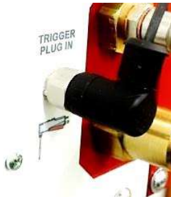
Fig. 8.7 Connection of oiling gun trigger
